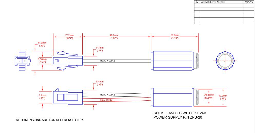
INPUT CONNECTOR MATES WITH JKL ZAF ALUMILINE LED SERIES LIGHT BARS.
