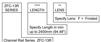
JKL Part Number Example: ZFC-13R1000-F Channel Series with 1 Meter (1000mm) Length and Frosted Lens.
