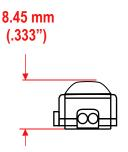
Note: Height is 8.98 mm (.35") with mounting tape attached
