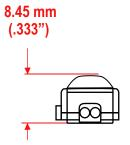
Note: Height is 8.98 mm (.35") with mounting tape attached
